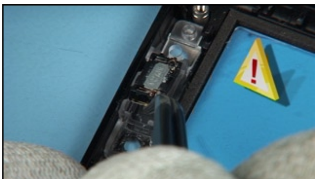
45. Ease out the EARPIECE from the shown side.
